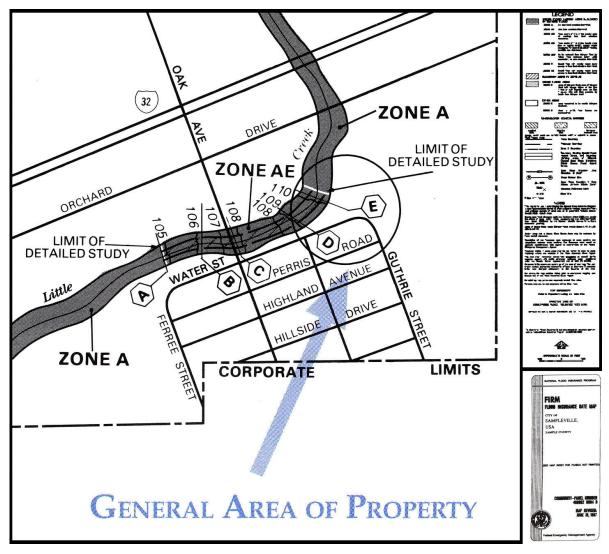
Figure 15. Sample Panel 0004 from a Z-fold Flood Map
